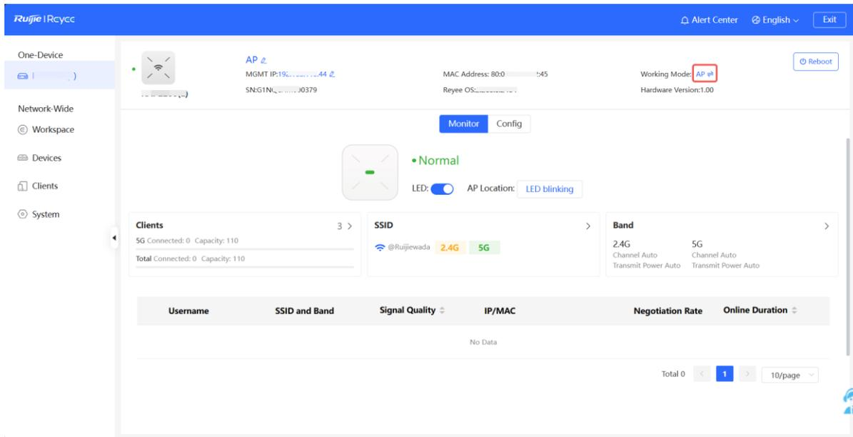
**AC function switch:** If a device works in the router mode and the self-organizing network discovery function is enabled, you can enable or disable the AC function. After the AC function is enabled, the device in the router mode supports the virtual AC function and can manage downlink devices. If this function is disabled, the device needs to be elected as an AC in self-organizing network mode and then manage downlink devices.
