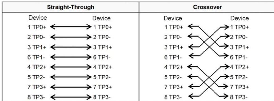
In addition to cables with the above-mentioned specifications, the 10BASE-T/100BASE-TX port can be connected using 100-ohm Cat3, Cat4, and Cat5 cables at 10 Mbps data speed or using 100-ohm Cat5 cables at 100 Mbps data speed with a maximum distance of 100 m (328.08 ft.). The following table shows 10BASE-T/100BASE-TX pin assignments.
