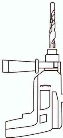
(2) Secure the mounting bracket to the ceiling or wall using wall anchors and Phillips pan head screws (M4 x 20 mm).
