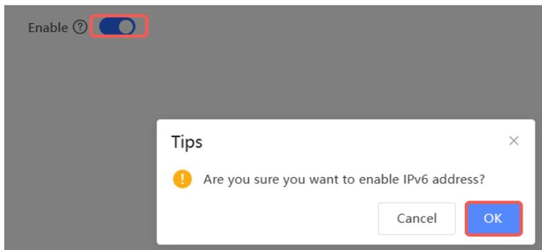
After IPv6 is enabled, you can configure the IPv6 addresses of WAN and LAN ports, view the DHCPv6 client, and configure a static DHCPv6 address for the client.
