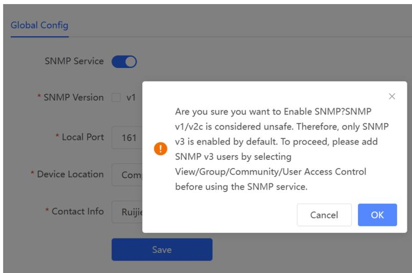
When it is enabled for the first time, SNMP v3 is enabled by default. Click **OK**.
